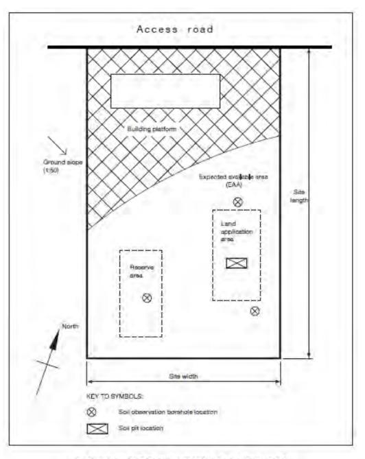
FIGURE D1 SITE PLAN - INDIVIDUAL LOT - EXAMPLE
