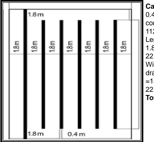
Calculation: 900L/d / 20mm/d / 0.4m (width of the standard concrete leach drain 400mm) = 112.5= 6 drains x 18.75m long Length of the LLA: 18.75m + 2 x1.8m (setback under Regs 1974) = 22.35mWidth of LAA= 0.4m (width of each drain) x 6 + 1.8m x 5 = 3.6m + 9m=15m22.35m x 15m = 335.25mTotal LAA=335sqm
