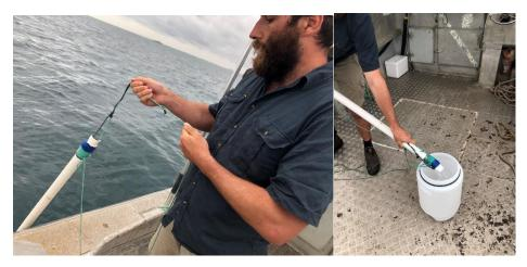
4. At those sites where the water depth is less than 2m and the water column is well mixed, a bucket with a rope attached should be used to collect the water sample. Avoid stirring up the sediment before sample collection. Collect at high or incoming tide. Mix the contents of the bucket and immediately fill the sample bottle to the neck by immersing the bottle in the bucket (see picture below). Do not allow the contents of the bucket to settle before filling the bottle.
